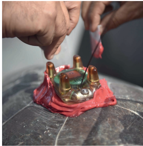
Attaching an Argos-GPS tag to the shell of a juvenile green turtle © DR
