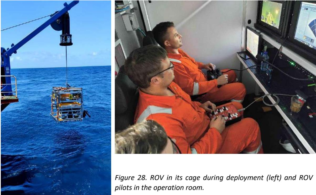
*Figure 28. ROV in its cage during deployment (left) and ROV pilots in the operation room.*
