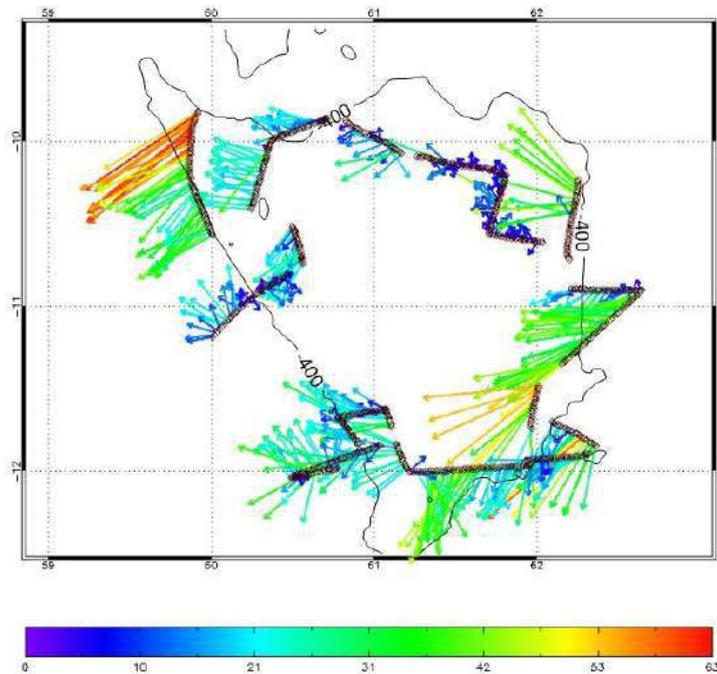
Figure 12. Current velocity (in cm s<sup>-1</sup>) and direction at 30 m measured by ADCP over Saya de Malha (delimited by isobaths -400 m), from 2 to 17 November 2022
