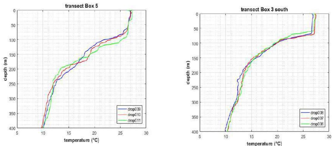
Figure 14. Left: Temperature profiles measured by 3 XTB launched on a transect perpendicular to the bank slope west of Saya de Malha (box 5): from the high sea (blue profile) to the bank slope (green profile). Right: same for 3 XBT on a transect east of Saya de Malha (box 3 south): from the high sea (blue profile) to the bank slope (green profile).
