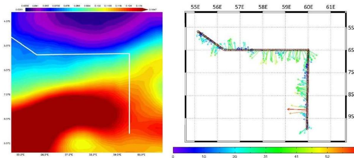
Figure 11. Left : Sea level anomalies (showing a cyclonic eddy in the north) with the ship track (white line) on the 1<sup>st</sup> November 2022. Right: Current velocity (in cm s<sup>-1</sup>) and direction at 30 m measured by the ADCP during the transit from Seychelles to Saya de Malha bank (31 Oct to 2 Nov).
