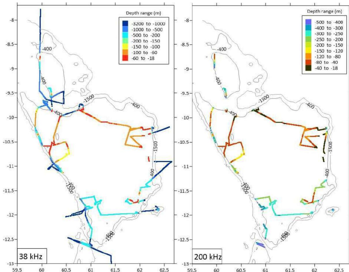
Figure 7. Depth measured by the SBES of the S.A. Agulhas II along sailing lines over the Saya de Maha Bank and outside its slopes. Two frequencies are shown to cover a large range of depths along the tracks.
