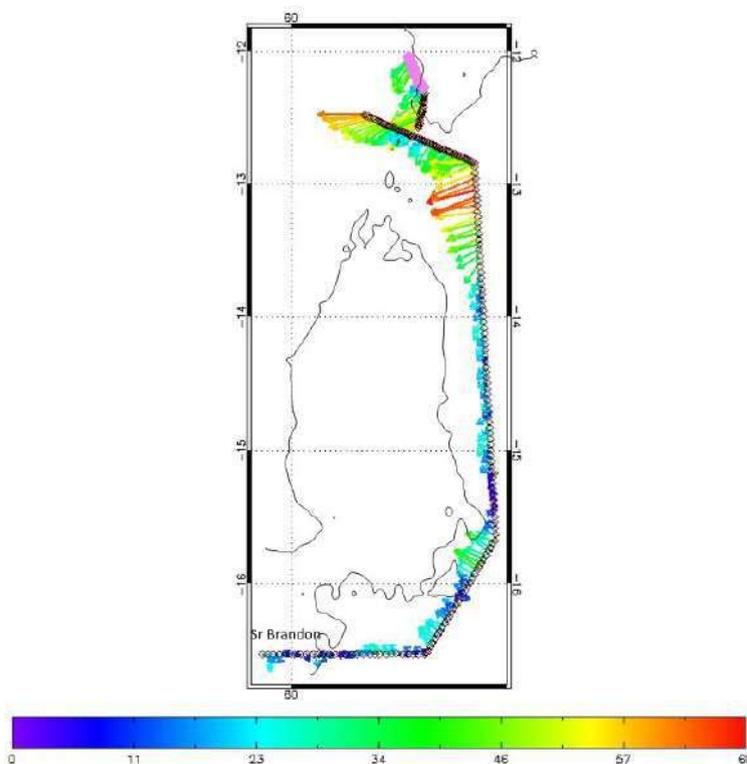
Figure 13. Current velocity (in cm s<sup>-1</sup>) and direction at 30 m measured by ADCP along the eastern edge of the Nazareth plateau (delimited by isobaths -400 m), from Saya de Malha to St Brandon, on 18 and 19 November 2022.
