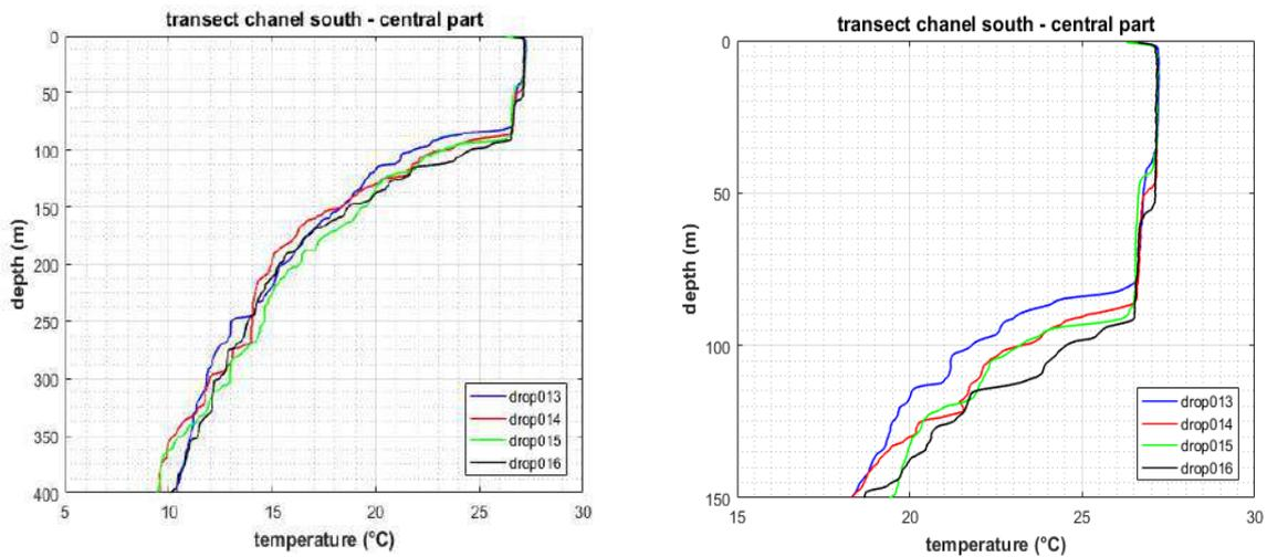
Figure 15. Left: Temperature profiles measured by 4 XBT launched on a transect crossing the channel between Saya de Malha and Nazareth banks, from west (drop013) to east. (drop016). Note that drop014 and drop 015 were above a relatively shallow topographic structure (about 400m depth). Right: same part of the transect with a zoom on the 0-150m upper layer.
